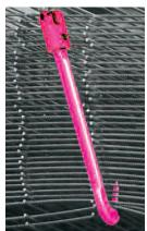
The bevelling on the back of the hook simplifies the horizontal hook insertion between the bales. The clevis connection enables a direct chain connection and the integrated ball bearing swivel prevents the chain from automatically spinning.
