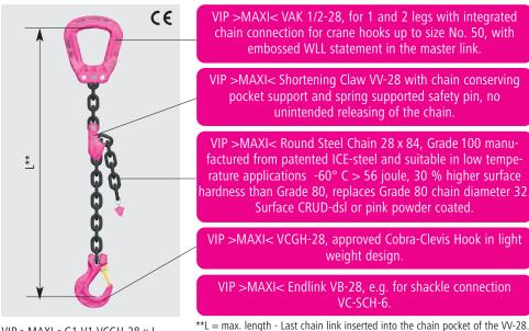
VIP >MAXI< VAK 1/2-28, for 1 and 2 legs with integrated chain connection for crane hooks up to size No. 50, with embossed WLL statement in the master link.
