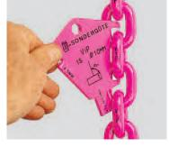
Testing for plastic elongation caused by overload
