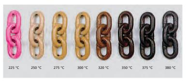
The special fluorescent VIP powder coating permanently shows the temperature to which the VIP chain has been exposed.
