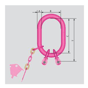
VBK 2 master link is supplied with two welded VRG connectors. Therefore only the correct chain diameter and number of legs can be connected. The identification tag with an integrated testing gauge is already attached. Connecting bolt and tensioning sleeve are pre-assembled.
